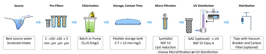
Pumps, valves, pipes, pressure tank, etc. omitted for clarity.
